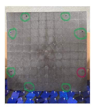
Check and sort all of your panels in this method and lay them face down on top of each other in a pile with all tops furthest away from you in the same position.
